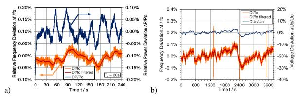
Figure 2: Measured frequency and calculated values on a capacitor with 300 Ws. a) Additional power flow. b) Voltage fluctuation,
