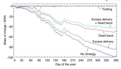
Figure 4: Effect of applying degrees of freedom for a battery storage with 1 MW rated Primary Control Power [14].
