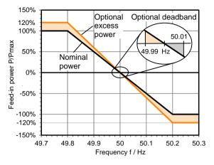
Figure 5: Degrees of freedom of the power delivery curve. According to [12].
