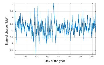
Figure 6: Calculated battery state of charge with frequency compensation using only a running average with an averaging length of one day for a battery storage with 1 MW rated Primary Control Power.
