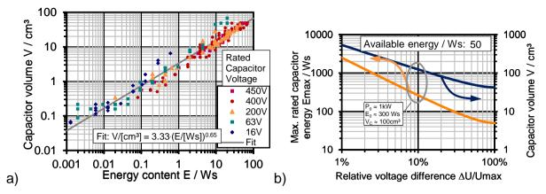
Figure 1: Volume size of electrolytic capacitors. a) Various electrolytic capacitors, data from [5]. b) Needed capacitor energy and volume size to store 50 Ws.
